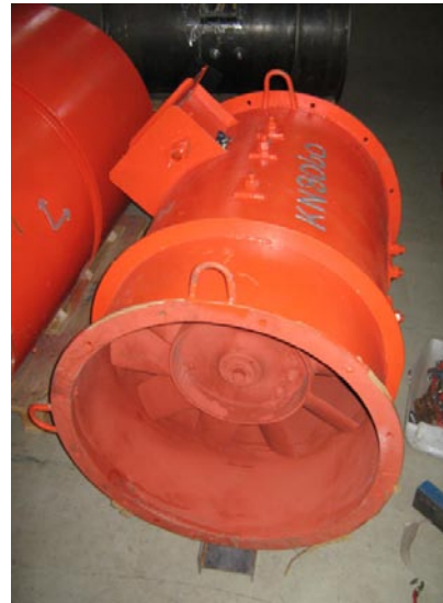
Figure 4: New axial ventilation fan
