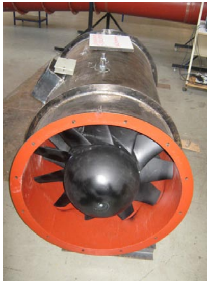
Figure 5: Existing steel axial ventilation fan
